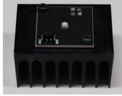
Picture 5. Fins facing down (This orientation obstructs the air flow)
